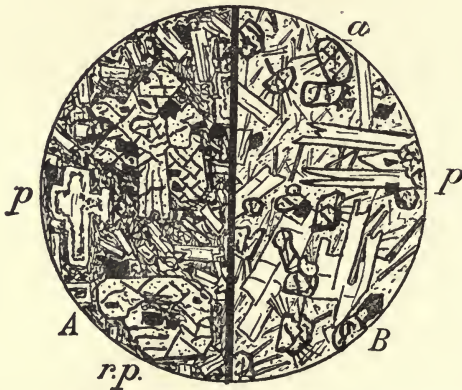
Fig. 36.— A , Pyroxene-Andesite (basaltic type). Kremnitz, Hungary. \times 14. p , Plagioclase. r.p. , Rhombic pyroxene (enstatite). Crystals of magnetite occur. Dark hemicrystalline groundmass. B , Glassy Pyroxene-Andesite (basaltic type). Dyke, Eskdale, Dumfries. \times 40. a , Granular augite, often set with radiating microlites from the glassy groundmass. p , Plagioclase in various stages of growth, often with characteristic bifurcating and incomplete terminations. Magnetite occurs. This rock exhibits the clear brown interstitial glass typical of many continental augite-andesites and "porphyrites."
